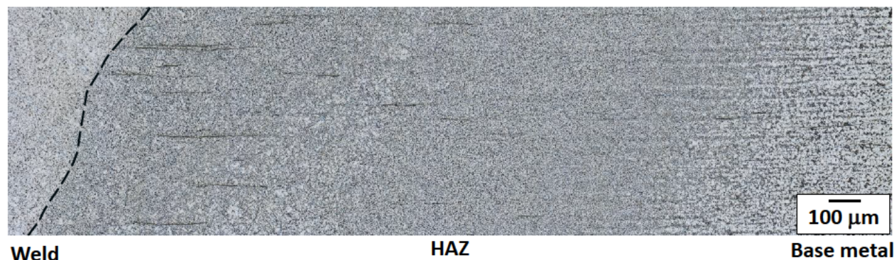
Figure 2: Etched cross section showing the weld fusion line and the variability of the microstructure in the HAZ of the X60A girth weld. The horizontally aligned features in the HAZ adjacent to the weld fusion line are MnS stringers.
